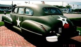
1942 Cadillac "Ike" staff car fully equipped Series 75, built by Fleetwood. In addition to the standard factory equipment that included a flathead V8, it has blackout shields for all of the lights, a siren and flag mounts. Everything on the outside is painted olive drab, including all of the chrome trim, hub caps, badging and hood ornament. It may be painted olive drab but the Cadillac crest and name is all over the car, every logo is intact.
